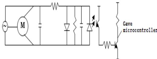
Figure 1. The Circuit of Pulse Detection
