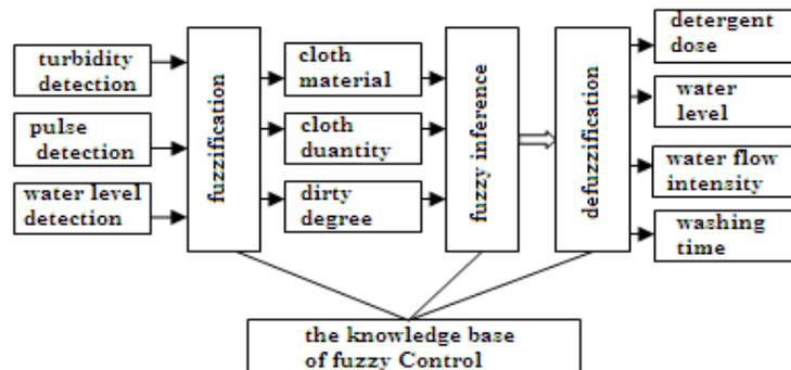
Figure 9. The Fuzzy Control Principle Diagram of the Intelligent Washing Machine
