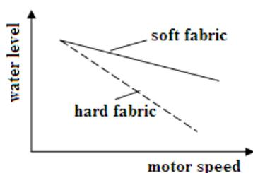
Figure 7. The Water Level Curve of Soft Fabric and Hard Thick Cloth
