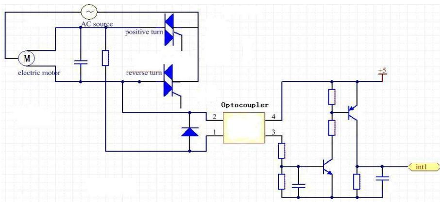
Figure 4. The Circuit Principle Diagram of Load Detection
