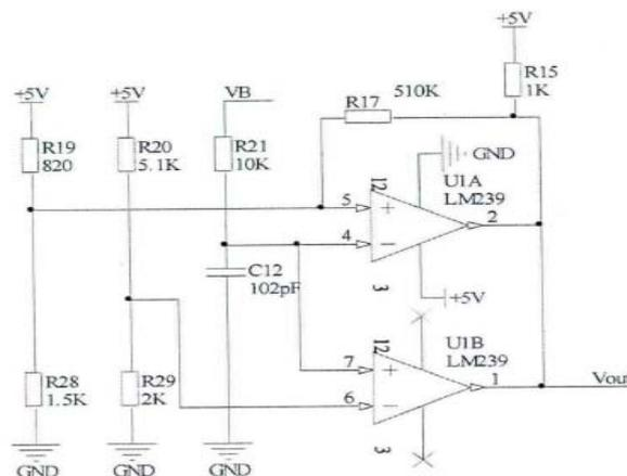
Figure 3. High and Low Voltage Protection Circuit
