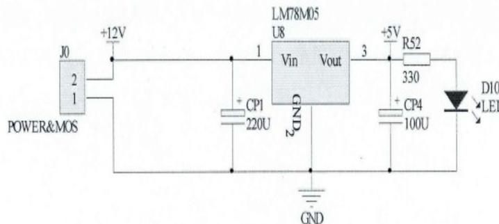
Figure 1. Power Supply Circuit
