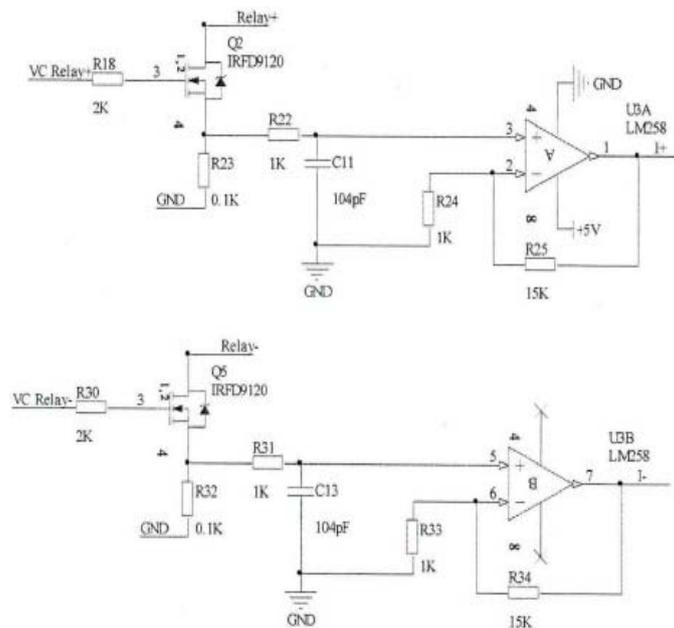
Figure 2. Positive and Negative End of the Relay Control and Current Sampling Circuit
