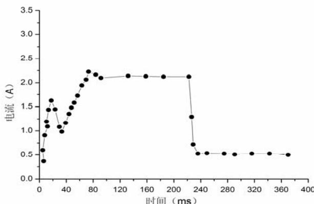
Figure 7. Closed for DC Contactor Coil Current Change Curve in the Process
