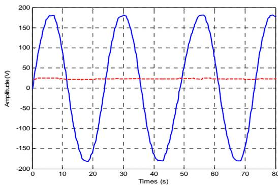
(a) Simulation wave with 100V (RMS) AC signal injected
