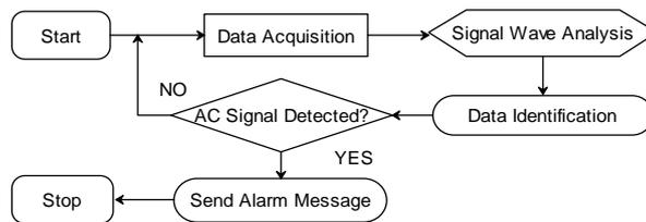
Figure 1. Flow Diagram of AC Signal Detection in DC Power System
