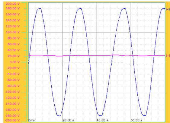
(b) Acquired wave with 100V (RMS) AC signal injected
