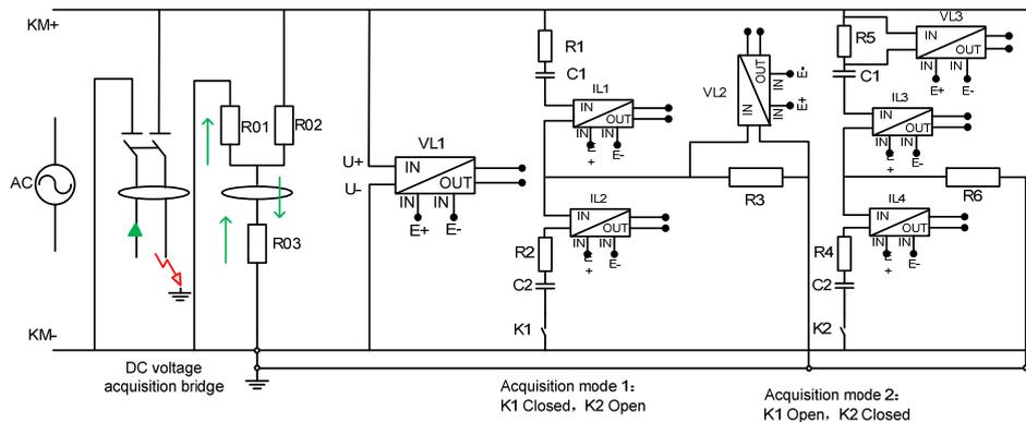
Figure 2. Schematic Diagram of AC Signal Detection in Positive and Negative Electrodes
