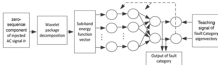
Figure 4. Structure of WNN for Fault Identification
