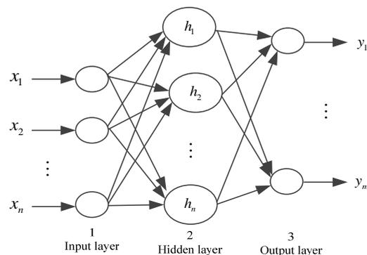
Figure 3. Topology of Wavelet Neural Network
