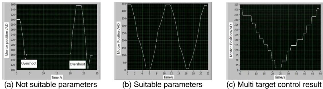
Figure 6. Result of Throttle Position PID Control Experiment
