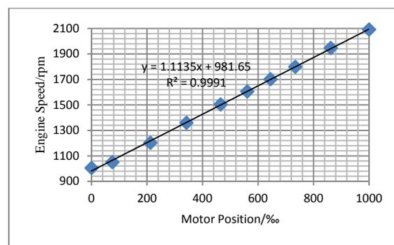
Figure 8. Curve between Throttle Position and Engine Speed
