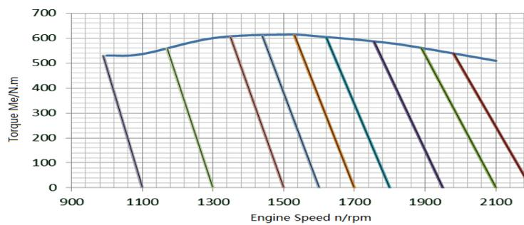
Figure 1. Govern Characteristics of Setting Engine Speed during Work
