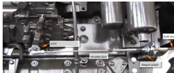
Figure 3. Connection of Speed Governor and Throttle Linear Motor
