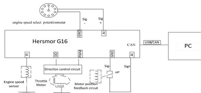
Figure 5. Engine Speed Control Circuit of Excavator
