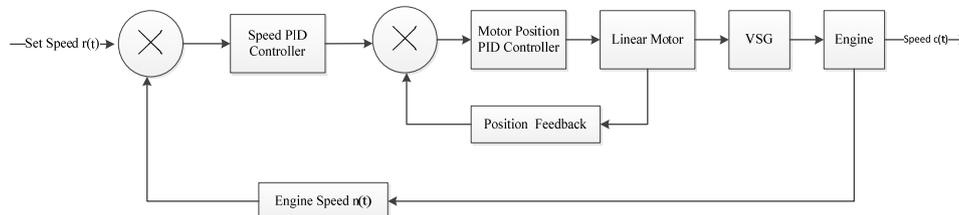
Figure 2. Double PID Control Model for Engine Rotation Speed of Excavator
