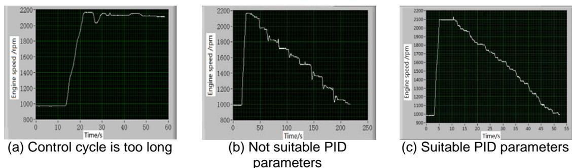
Figure 7. Engine Speed Control Result Based on Speed and Throttle Motor Position with Segment-PID Method
