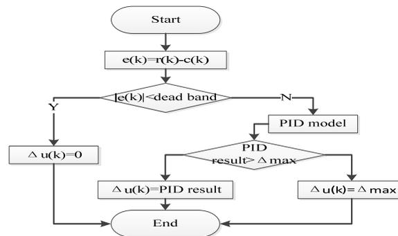
Figure 4. Incremental PID Method with Dead Band Zone and Maximum Increment Limit
