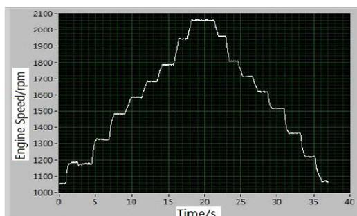
Figure 9. Engine Speed Following with Throttle Switch
