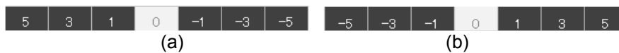
Figure 7. Masks for Detecting (a) Leftmost Position and (b) Rightmost Position of the Outer Boundary
