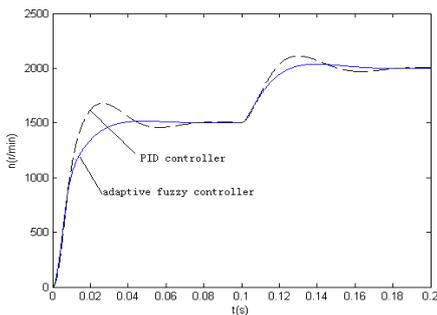
Figure 6. Speed Response with Step Change in Reference Speed (J=0.0012kg.m<sup>2</sup>)
