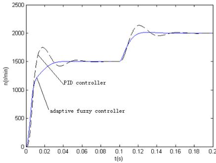
Figure 4. Speed Response with Step Change in Reference Speed
