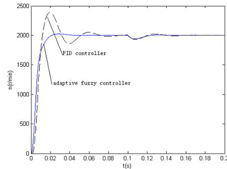
Figure 5. Speed Response with Step Change in Load Torque
