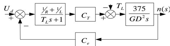
Figure 1. The BLDC Motor Dynamic Structure
