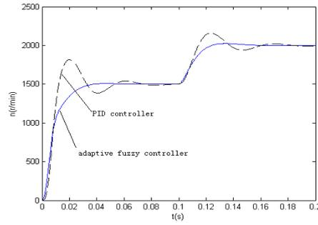
Figure 7. Speed Response with Step Change in Reference Speed (J=0.002kg.m<sup>2</sup>)
