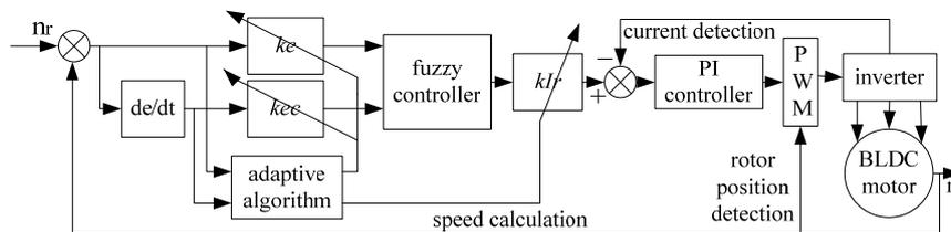
Figure 2. Control System Structure of the BLDC Motor
