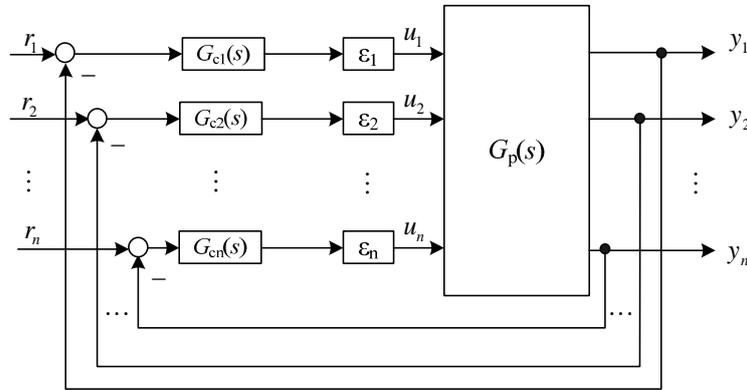
Figure 1. MIMO Control System Considering Integrity
