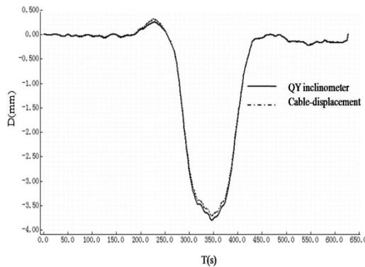
Figure 7. The Dynamic Deflection Curve of 25 meter Point when Train Runs Across with 5Km/h speed
