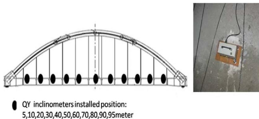
Figure 6. Installing Positions of QY Inclinometers
