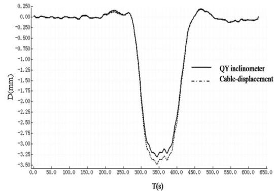
Figure 8. The Dynamic Deflection Curve of 50 meter Point when Train Runs Across with 5Km/h Speed
