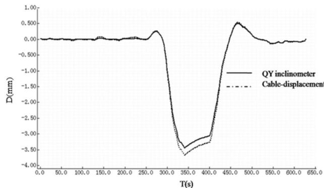
Figure 9. The Dynamic Deflection Curve of 75 meter Point when Train Runs Across with 5Km/h Speed
