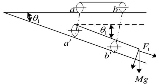
Figure 3. The Force Balance of YQ Inclinometer
