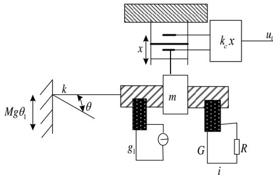
Figure 2. The Structure Principle of QY Inclinometer
