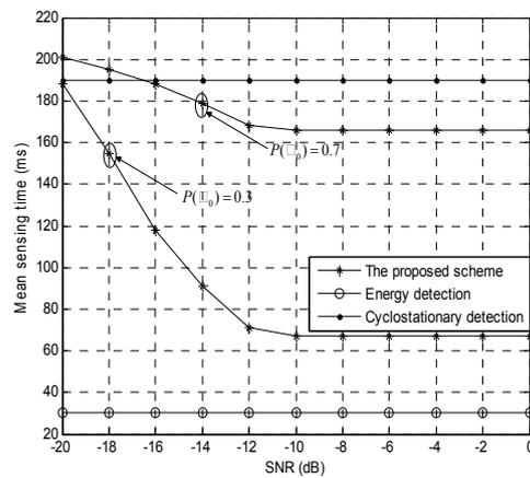
Figure 4. Mean Sensing Time versus SNR for Different Sensing Scheme
