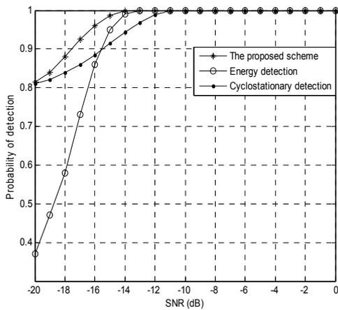
Figure 3. Probability of Detection versus SNR for Different Sensing Scheme
