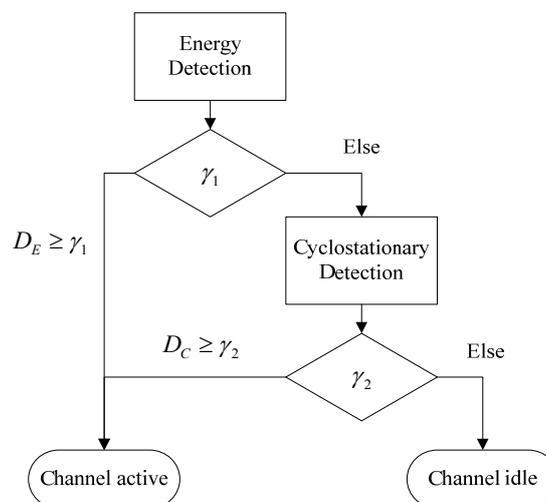
Figure 1. Adaptive Two-stage Spectrum Sensing
