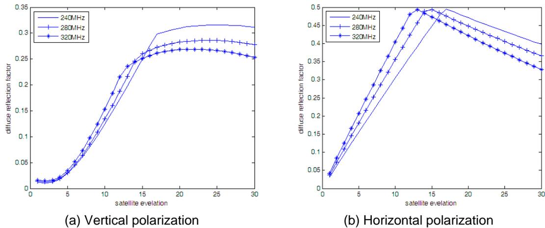
Figure 4. Diffuse Reflection Factor in Different Polarization Modes
