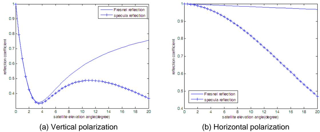
Figure 3. Fresnel and Specular Reflection Coefficient in Different Polarization Modes
