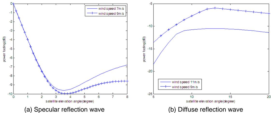
Figure 5. Power Fading of Specular and Diffuse Reflection Wave Relative to Direct Wave in Different Wind Speeds
