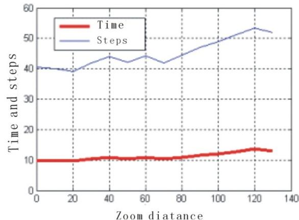
Figure 4. Time and Steps Cost by Auto-focus Process at Different Initial Position
