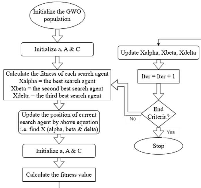
Figure 5. Flowchart showing the working of algorithm for GWO
