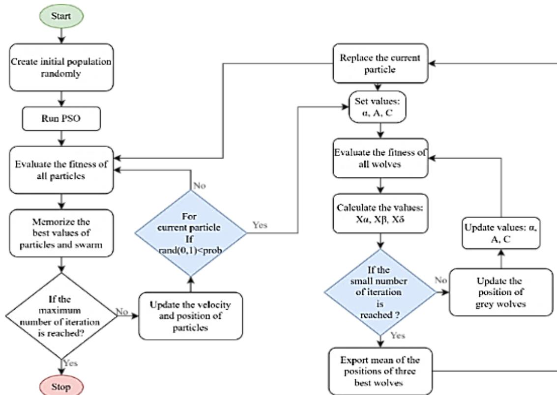
Figure 8. Flowchart for the working of hybrid GWO-PSO algorithm
