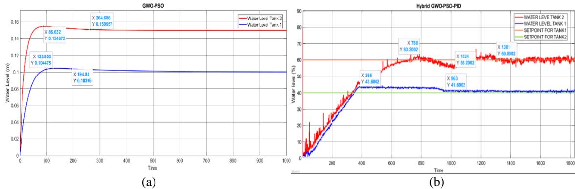
Figure 9. Response for water level control in coupled tanks using hybrid GWO-PSO-PID controller for (a) simulation and (b) hardware
