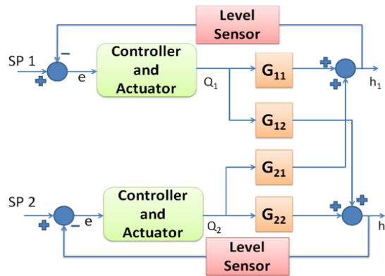
Figure 3. Block diagram representation of two tank interactive liquid level control system
