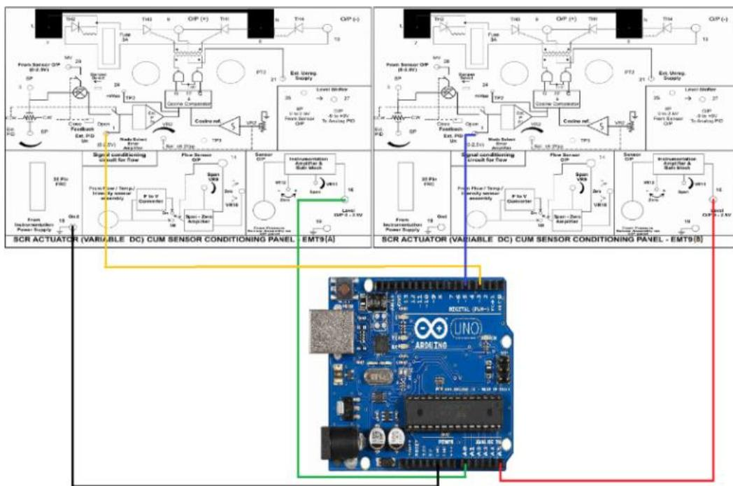
Figure 2. Circuit diagram for interfacing of controller kit with Arduino Uno
