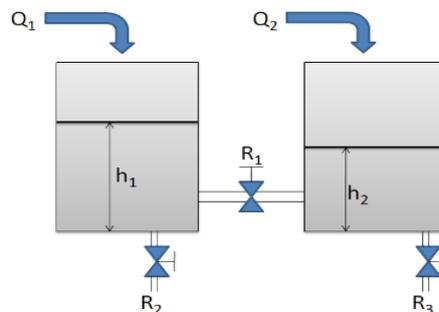
Figure 1. Schematic of coupled tanks
