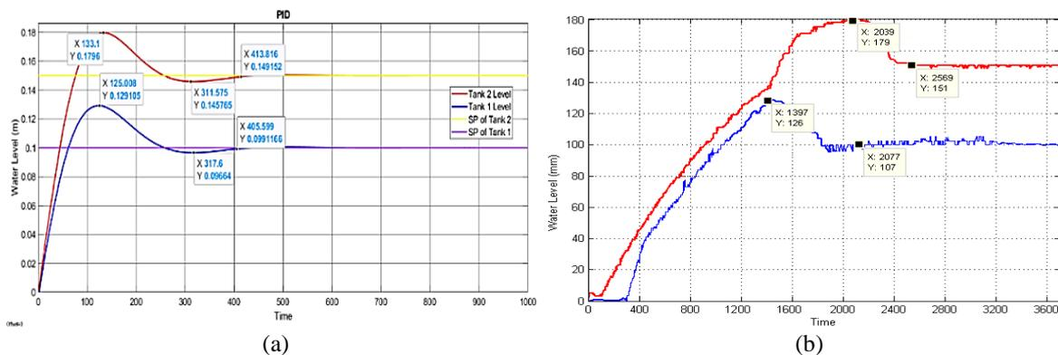
Figure 4. Response of water level in coupled tanks using PID controller for (a) simulation and (b) hardware
