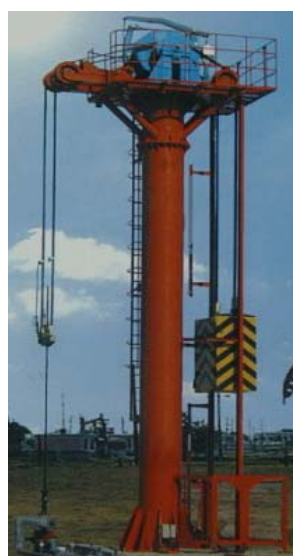
Figure 1. Direct Drive Pumping Unit
