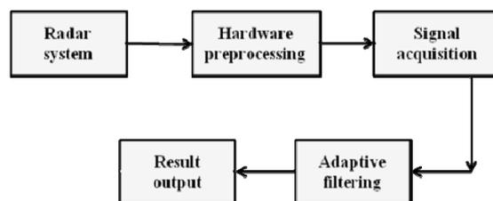
Figure 3. A Block Diagram of Non-Contact Bio-Radar Vital Signs Detection System
