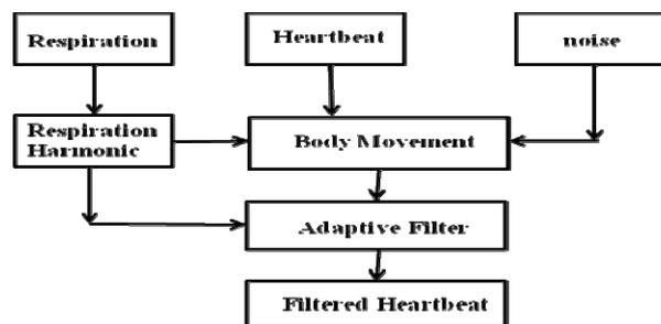
Figure 2. Adaptive Harmonic Cancellation Algorithm Based on LMS
