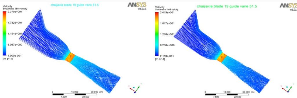
Figure 3. The Flow Pattern in the Full Hydraulic Duct of the Unit When Head of 5.5m And 6.5m
