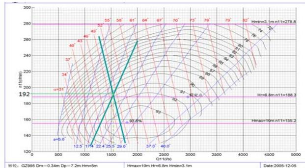
Figure 2. The Combined Characteristic Curve of the Bulb Turbine
