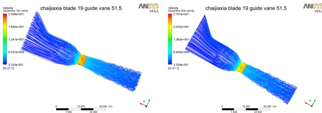
Figure 4. The Flow Pattern in the Full Hydraulic Duct of the Unit When Head of 7.0m And 7.5
