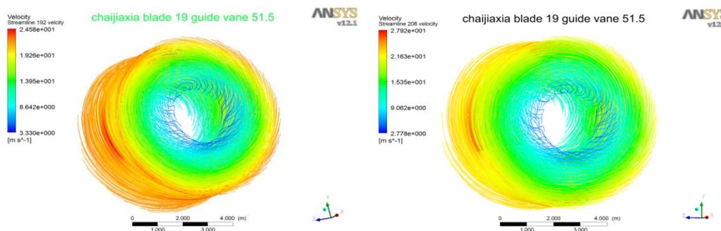
Figure 5. The Flow Patternn in the Outlet of the Runner When Head of 7m And 7.5m
