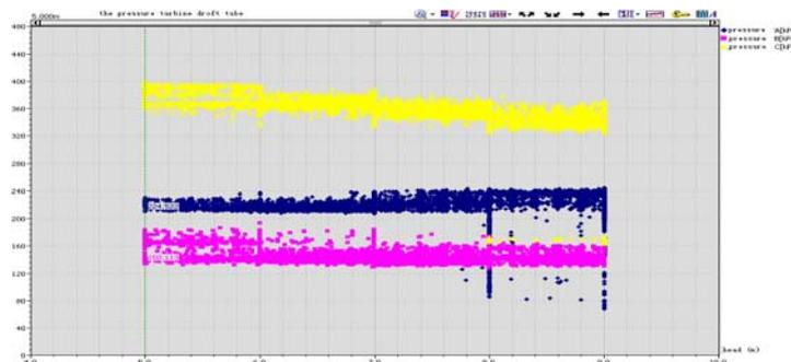
Figure 11. The Pressure Pulsation of the Turbine Draft Tube after Increasing Effective Water Head
