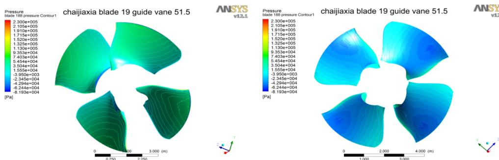
Figure 8. The Pressure Distribution on the Front and Back of the Runner Blade When Head of 6.0m
