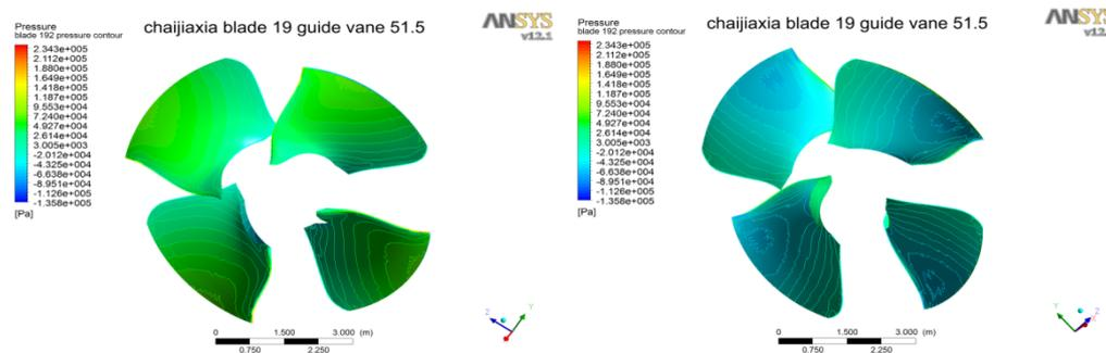
Figure 9. The Pressure Distribution on the Front and Back of the Runner Blade When Head of 7.0m
