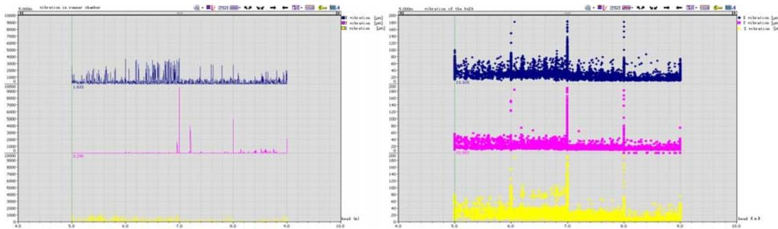
Figure 12. The Vibration of the Runner Chamber and Bulb after Increasing Effective Water Head
