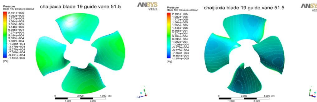
Figure 7. The Pressure Distribution on the Front and Back of the Runner Blade When Head of 5.5m
