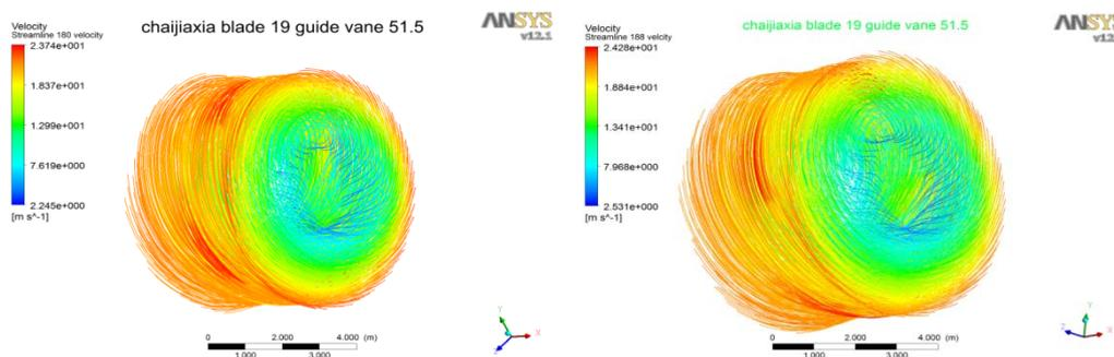
Figure 5. The Flow Patternn in the Outlet of the Runner When Head of 5.5m And 6.5m
