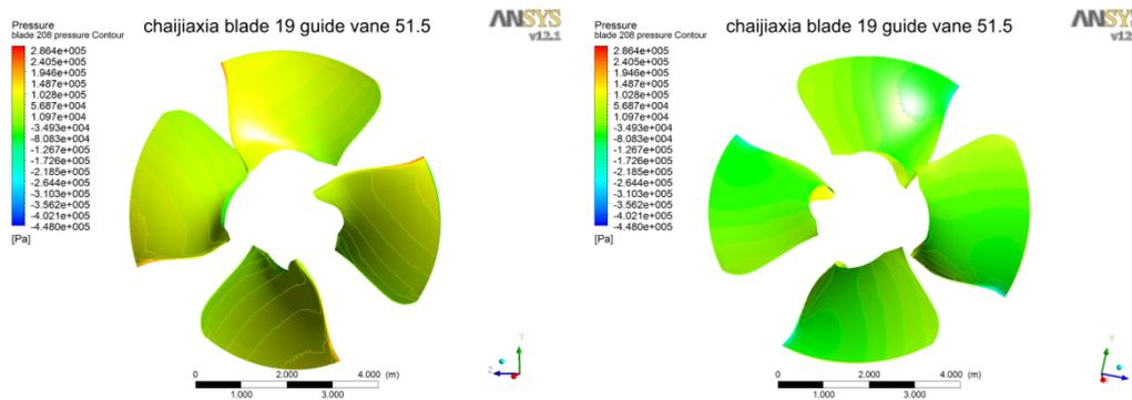
Figure 10. The Pressure Distribution the Runner Blade When Head of 7.5m
