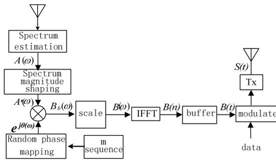
Figure 1. Principle Diagram of TDCS Transmitter
