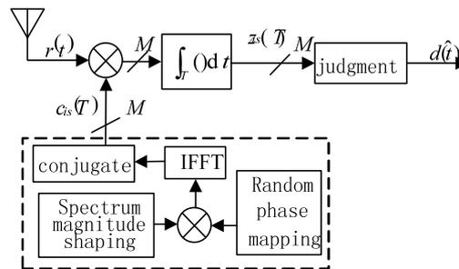
Figure 2. Principle Diagram of TDCS Receiver
