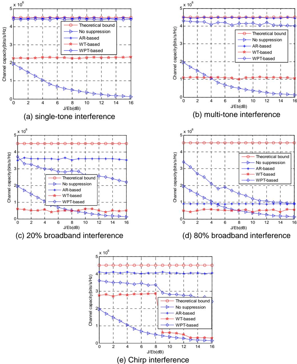
Figure 3. TDCS Channel Capacity under Different Spectrum Energy Detection Methods
