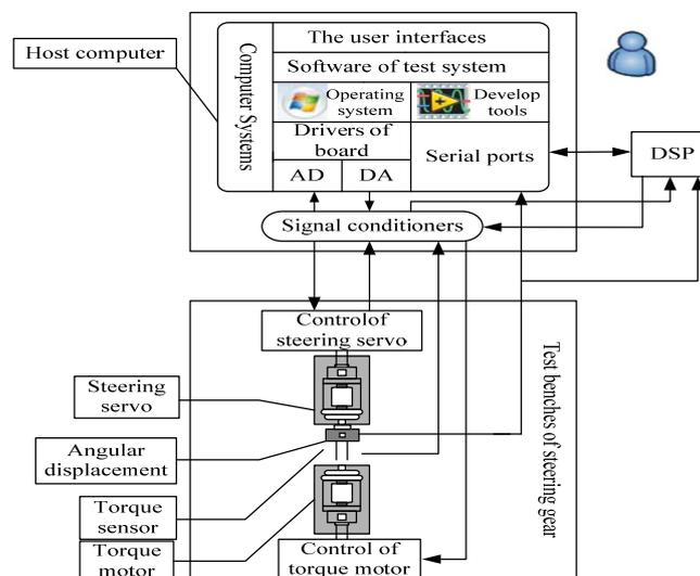
Figure 2. Overall Structure Diagram of Measuring System
