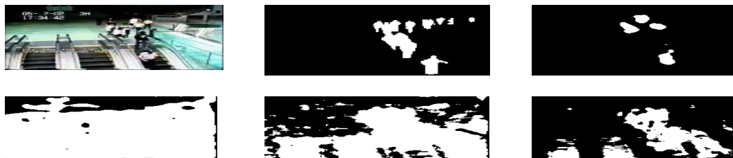
Figure 6. Escalator Video: (a) current frame; (b) Ground Truth foreground Mask; (c) MoGv2; (d) GMG; (e) Texture BGS; (f) Proposed method
