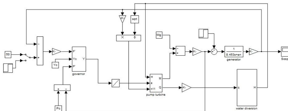
Figure 10. Simulation Model of Regulating System of Plant B
