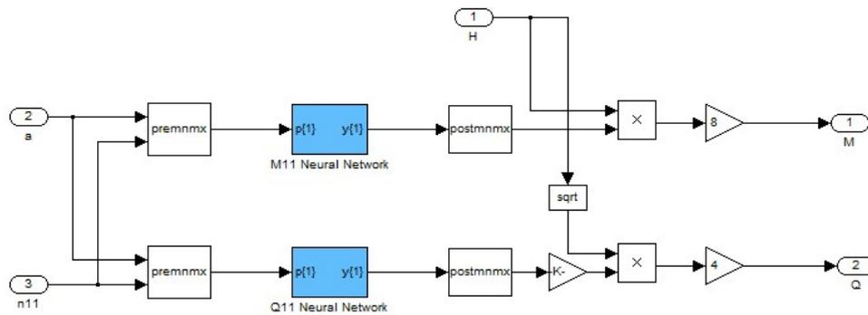
Figure 9. RBF Network Based Simulation Model of Pump Turbine
