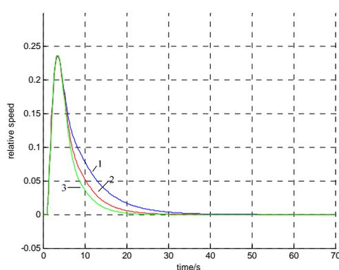
Figure 13. Comparison of Optimization Results of Load Shedding Process
