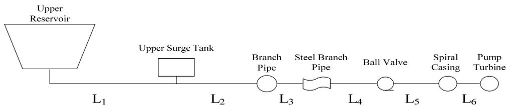
Figure 2. Diagram of Diversion System of Plant B (single penstock-single turbine)
