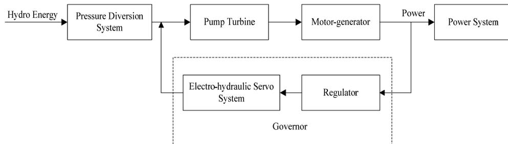
Figure 1. Structure of Regulating System of Pumped Storage Unit
