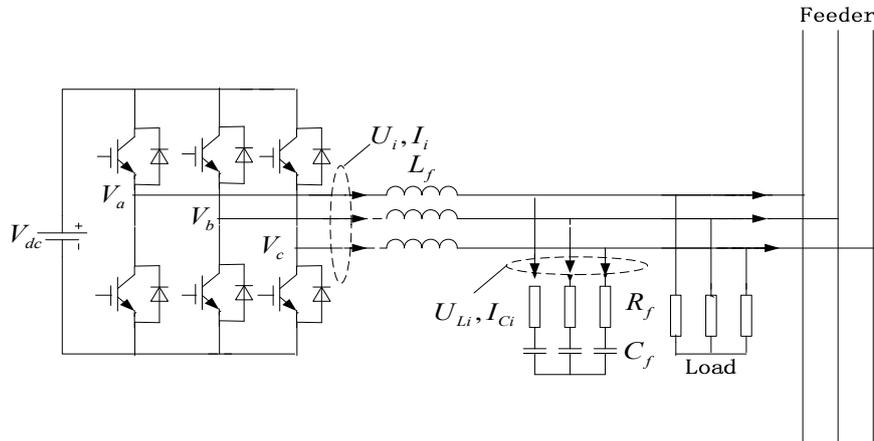
Figure 4. Circuit Structure of Three-phase Inverter
