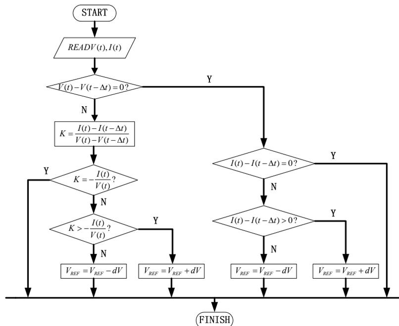
Figure 3. Flow Chart of the Incremental Conductance Algorithm
