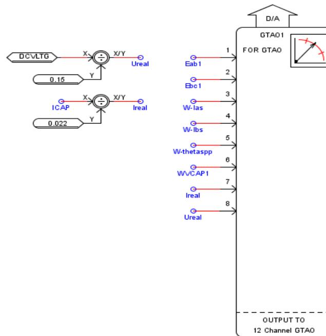
Figure 8. Setup of GTA0 Card in RTDS
