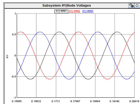
Figure 10. Grid-connect Voltage of Hybrid PV System
