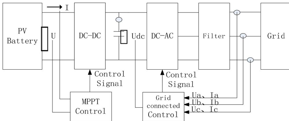
Figure 1. PV Grid-connected Power Generation System
