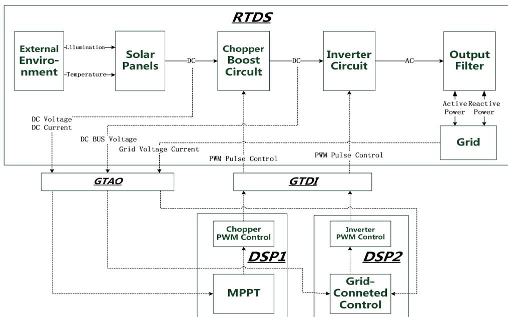
Figure 6. Framework of Hardware-in-loop Simulation System
