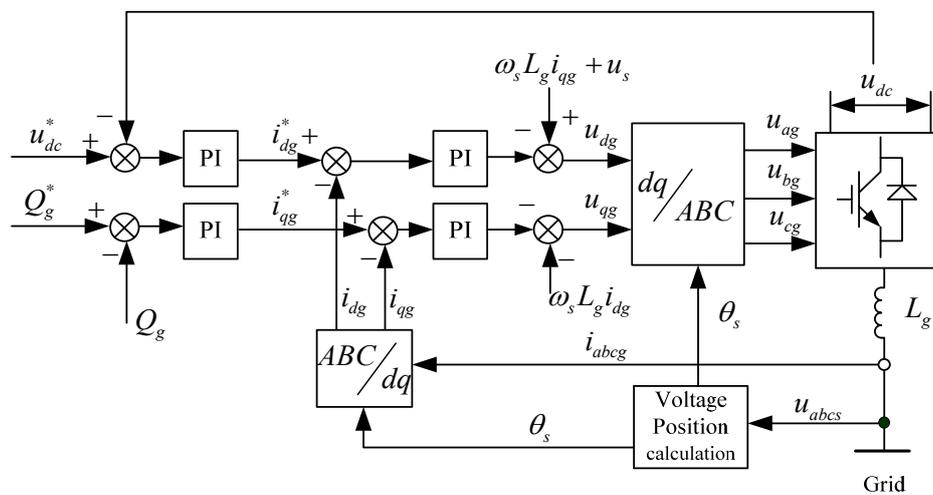
Figure 5. Schematic Diagram of a Three-phase Inverter
