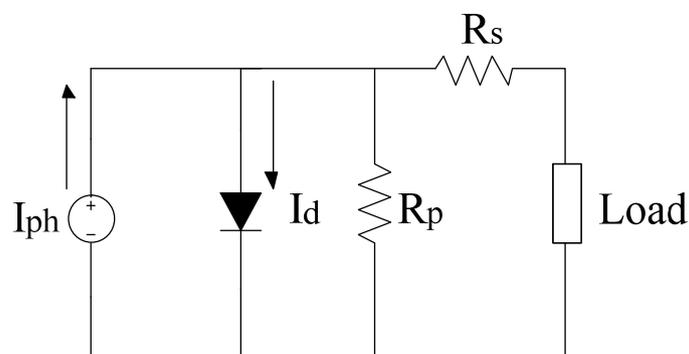
Figure 2. Equivalent Circuit of PV Battery
