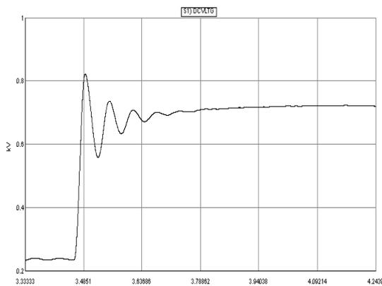
Figure 9. Voltage of PV Array when MPPT Starts
