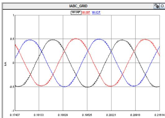
Figure 11. Grid-connect Current of Hybrid PV System
