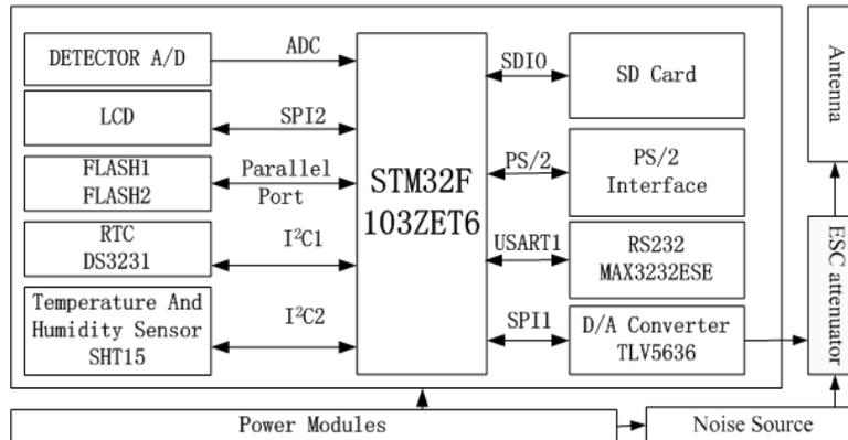
Figure 2. Embedded System Functional Block Diagram
