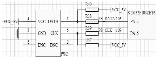
Figure 7. PS/2 Interface Circuit
