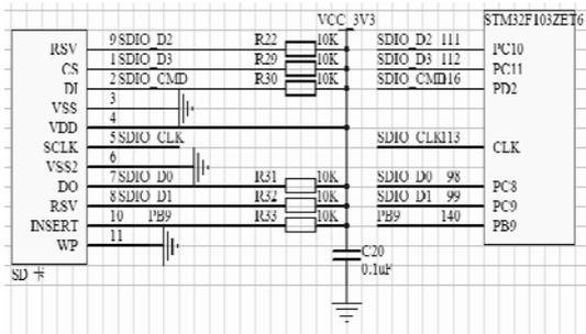
Figure 8. SD card Interface Circuit
