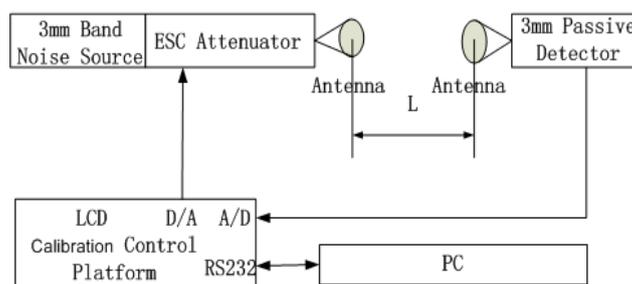
Figure 1. 3mm Band Calibration Platform System
