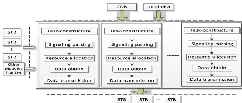
Figure 4. Full Parallel Architecture for Video Streaming with Multi-core Platform
