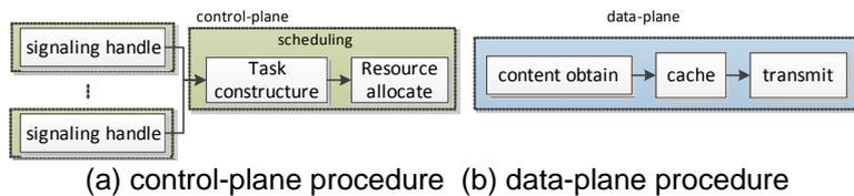
Figure 3. Detail of Pipeline-parallel Hybrid Architecture
