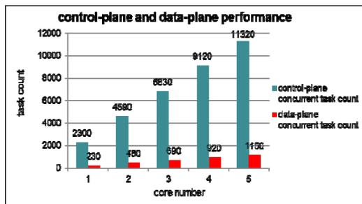
Figure 8. Task Number per Core Using openMP
