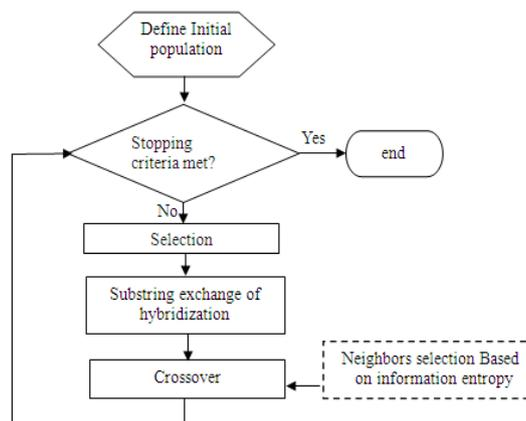
Figure 1. Heuristic Genetic Algorithm Flowchart
