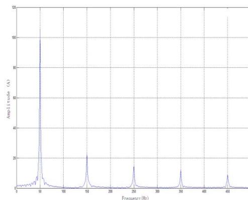
Figure 6. Electric Locomotive Reactive Power      Figure 7. Harmonic Content Analysis Diagram
