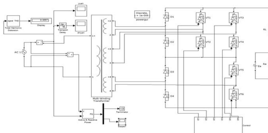
Figure 2. Simulation Model of  $ss_8$  Electric Locomotive
