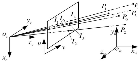
Figure 1. Point Pinhole Imaging Model
