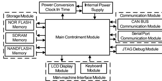
Figure 1. The Hardware Framework of PLC Editor System
