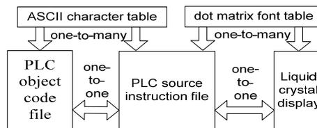
Figure 3. The Mapping Relation among PLC Source Instruction File, Object Code File, the ASCII Character Table and Dot Matrix Font Table
