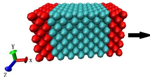
Figure 3. A 3D Ideal Cu Crystal, left and right boundaries are shown in red, arrow points the loading direction (the figure is done by molecular visualization program - VMD)
