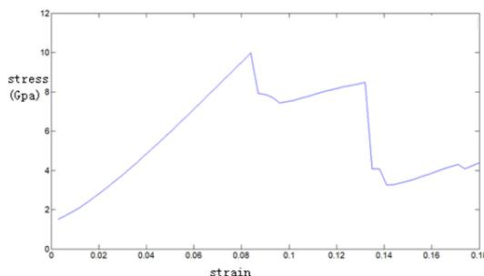
Figure 6. The Stress-Strain Curve of Crystal Copper during Tension Process by Molecular Statics Method
