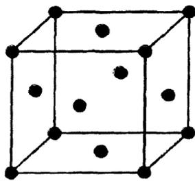
Figure 2. The Crystal Lattice of Cu
