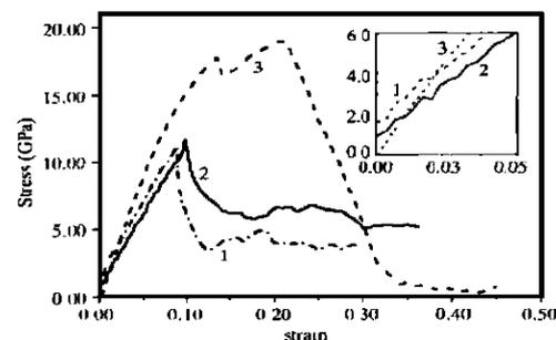
Figure 7. Stress-Strain Curve of Single Crystal Copper during Tension Process by Molecular Dynamic Method [13]
