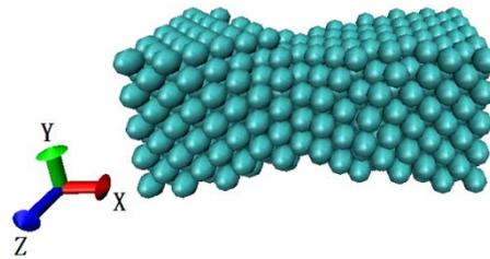
Figure 5. Strain  $\varepsilon=30.0\%$ , the Model Shape During the Plastic Deformation
