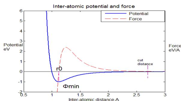
Figure 1. Interatomic Potential Energy and Force
