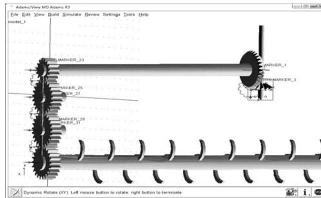
Figure 3. Virtual Prototype for the Drivetrain of Reversal Stubble-breaking Rototiller with All Constraints
