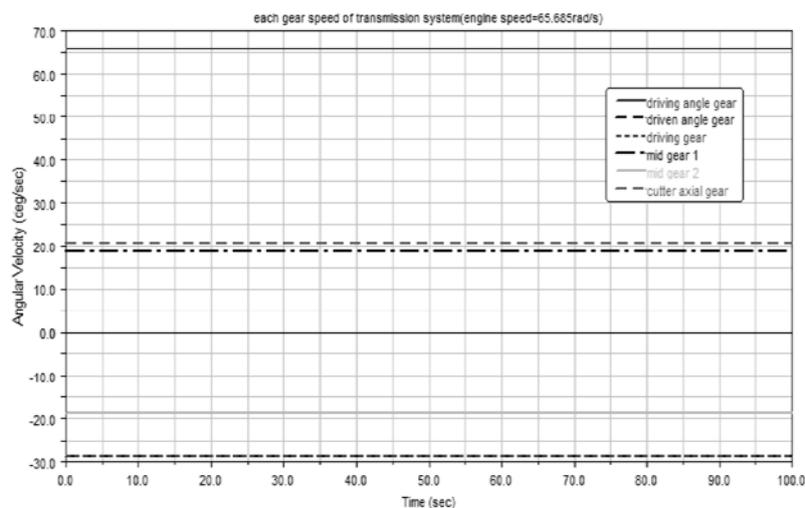
Figure 4. The Rotational Speed Simulation Graph of Each Drivetrain Gear at Engine Speed of 65.685rad/s
