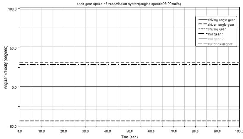
Figure 5. The Rotational Speed Simulation Graph of Each Drivetrain Gear at Engine Speed of 98.99rad/s
