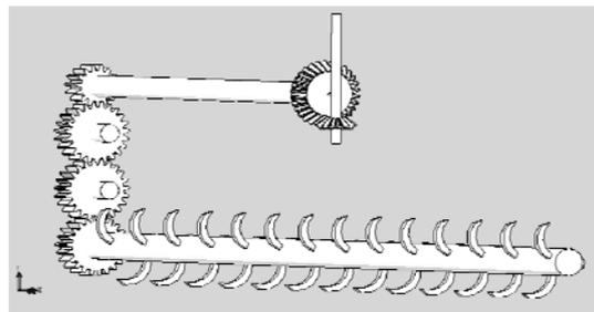
Figure 2. Virtual Assembly Drawing of the Drivetrain of Reversal Stubble-breaking rototiller
