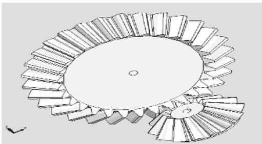
Figure 1. Meshing Model of the Driving and Driven Bevel Gear
