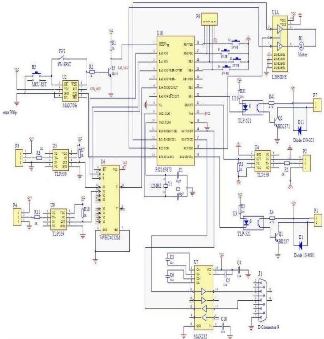
Figure 2. PIC Control Circuit of Cutting Machine
