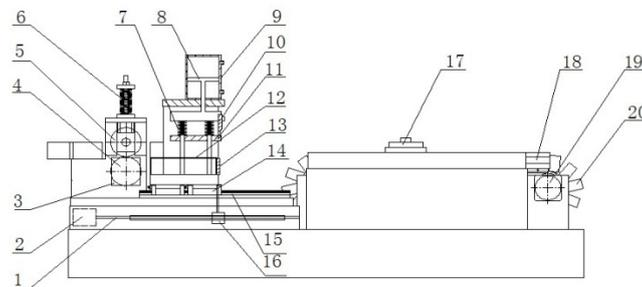
1 ball screw 2 walking motor 3 wheel motor 4 lower wheel 5 upper wheel 6 upper roller spring 7 rag iron spring 8 piston 9 cylinder 10 upper cutter 11 vermicelli platen 12 vermicelli picking plate 13 fixed lower cutter 14 walking slider 15 linear rolling guide 16 screw nut 17 sensor 18 sensor walking motor 19 production line motor 20 production line belt conveyor
