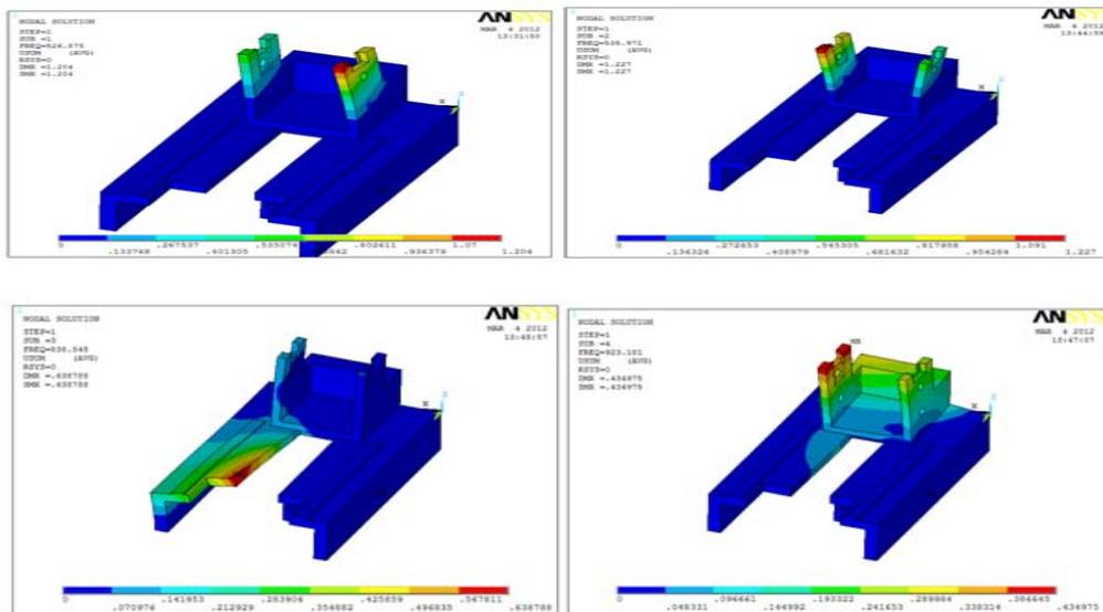
Figure 6. Deformation Diagram of 1-4 Order Nature Frequency for the Support
