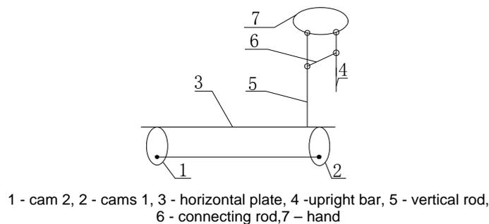
Figure 3. Structure Diagram of Flip Motion
