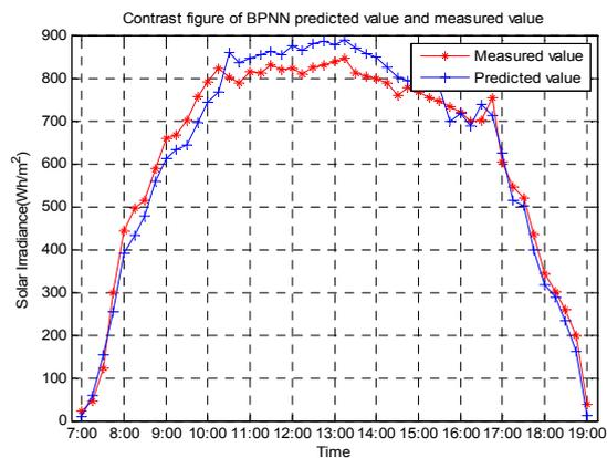
Figure 6. Result Comparison of Irradiance Predicted by BPNN
