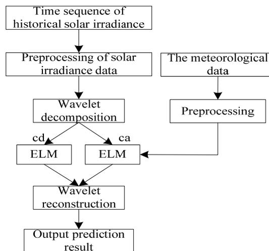
Figure 3. Block Graph of Solar Irradiation Prediction Process
