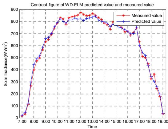
Figure 5. Result Comparison of Irradiance Predicted by WD-ELM
