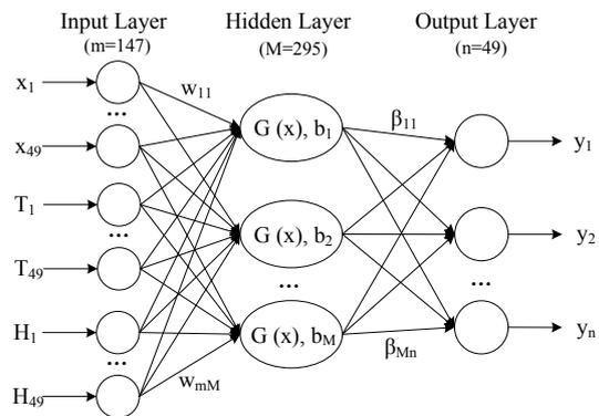
Figure 2. Prediction Model of Detail Composition
