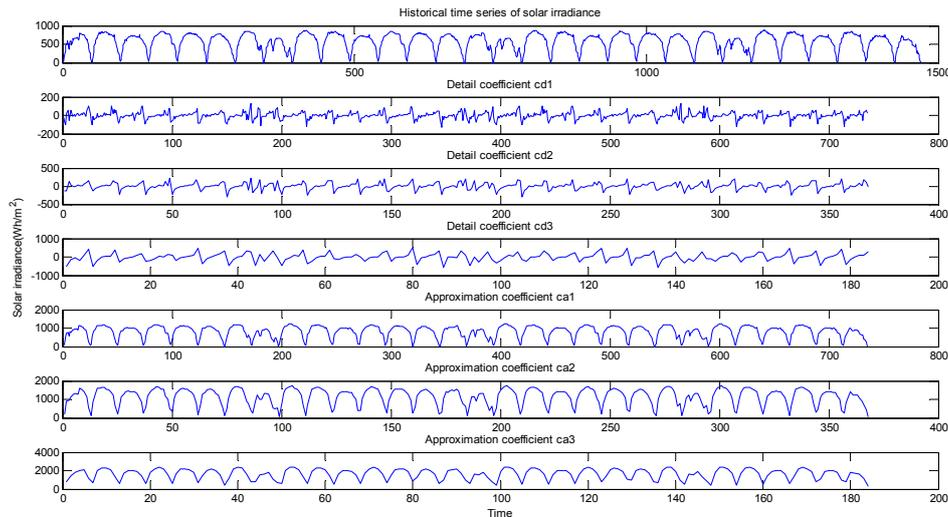
Figure 4. Wavelet Decomposition of Solar Irradiance in One Month
