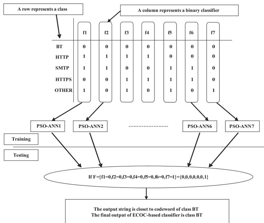
Figure 1. Training and testing phases of the ECOC-based odel
