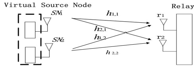
Figure 2. Virtual VBLAST Model of Multiple Access Stage
