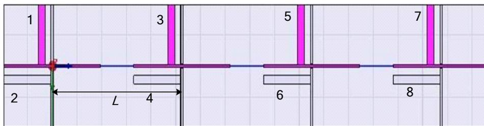
Figure 7. Geometry of the Proposed Horizontal/Vertical Dual-polarized Antenna
