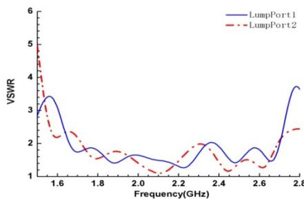
Figure 10. VSWR of Dual-polarized Antenna Array
