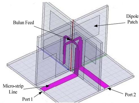
Figure 2. Simulation Structure Diagram of the Dual-polarized Antenna
