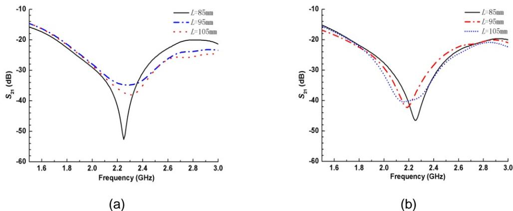
Figure 8. Isolation between port1 and port2, port3 and port4 with different value of  $L$
