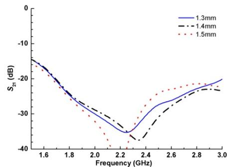
Figure 5. Isolation with Different Height of the Slot
