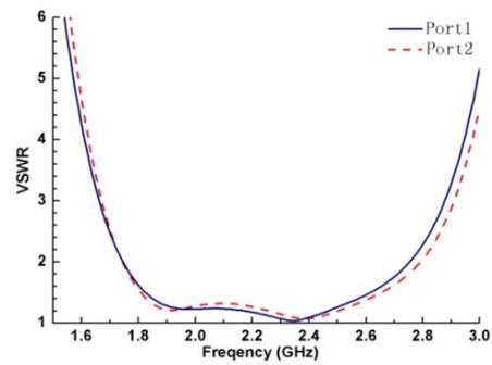
Figure 3. VSWR of Dual-polarized Antenna
