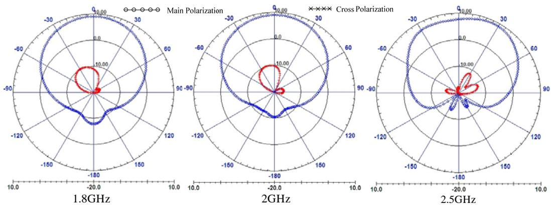
Figure 6. Horizontal Radiation Pattern of Dual-polarized Antenna
