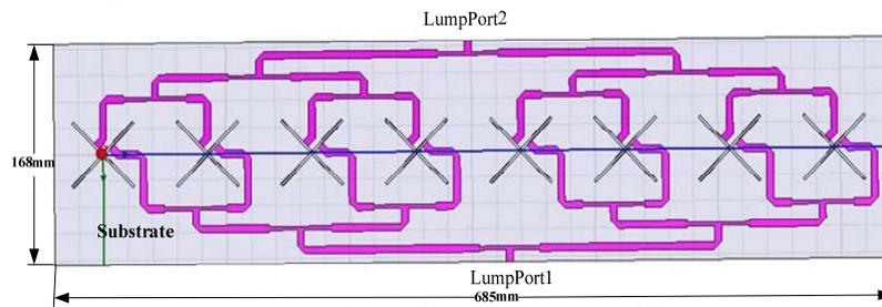
Figure 9. Geometry of the Proposed 8-unit Dual-polarized Antenna Array of  $+45^\circ/-45^\circ$  Polarization
