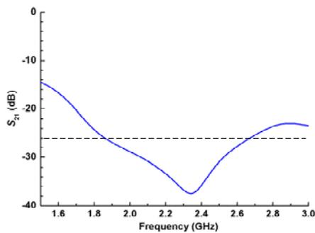
Figure 4. Isolation of the Dual-polarized Antenna
