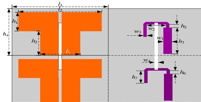
Figure 1. Geometry of the Proposed Dual-polarized Antenna
