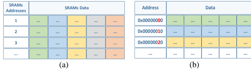
Figure 4. Database arrangement using (a) conventional SRAMs and (b) the proposed SDRAM method
