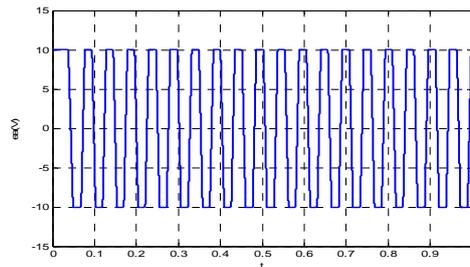
Figure 4. A Reverse Electromotive Force Response Curve
