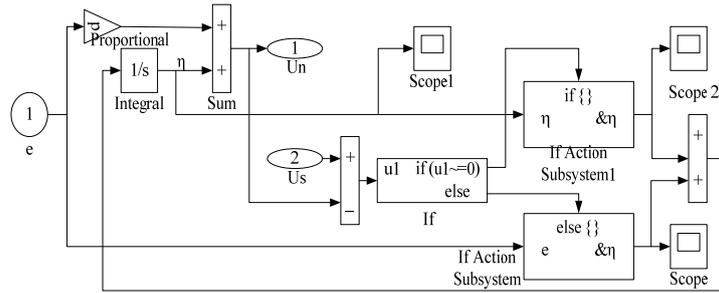
Figure 1. Anti-windup PI Controller Model
