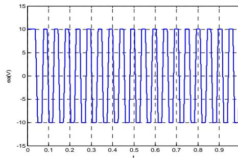
Figure 7. A Reverse Electromotive Force Response Curve
