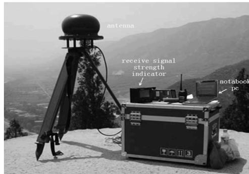
Figure 7. The Ground Receiving Equipment
