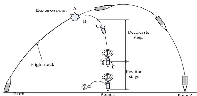
Figure 3. Schematic Diagram of the Rocket and Memory Flight Path
