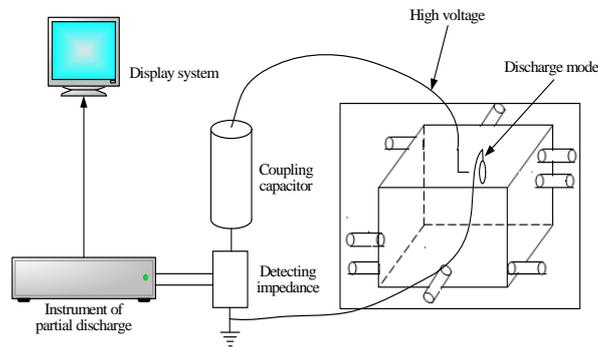
Figure 5. The Measurement Principle of the Partial Discharge
