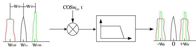
Figure 6. The Changes in the Spectrum After Mixing One Way of Frequencies
