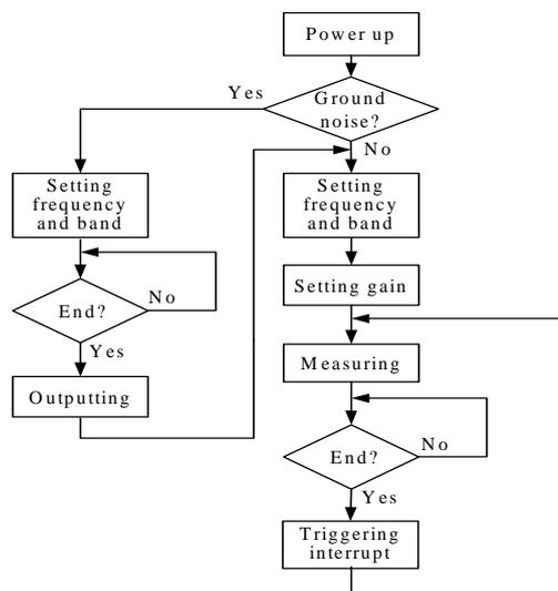
Figure 8. The Monitoring Program Workflow of the Acquisition Card
