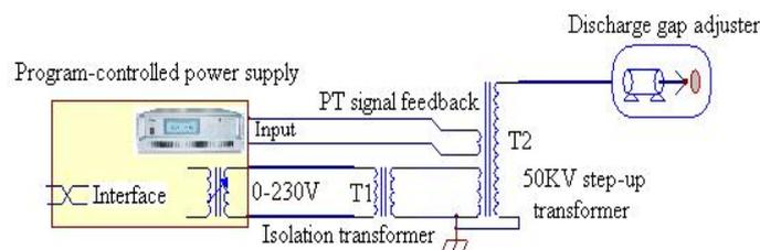
Figure 4. The Control Principle of the Discharge Voltage
