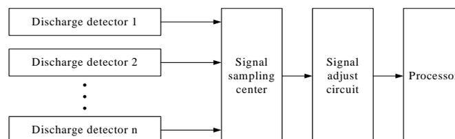
Figure 2. The Functional Block Diagram for the Monitoring System
