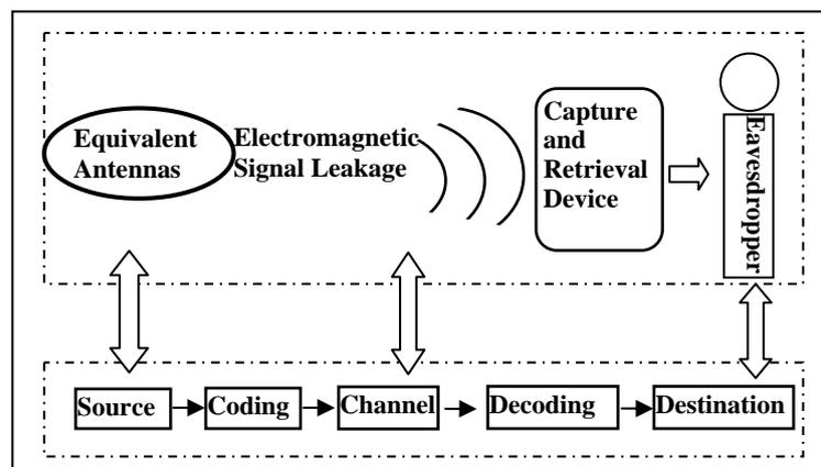
Figure 1. Diagram of Model for Electromagnetic Information Leakage
