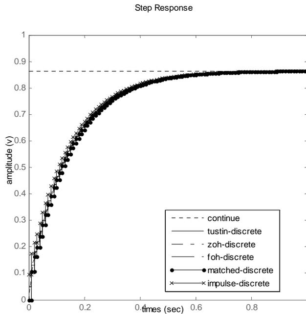
Figure 8. Comparison step response of discrete system with several methods
