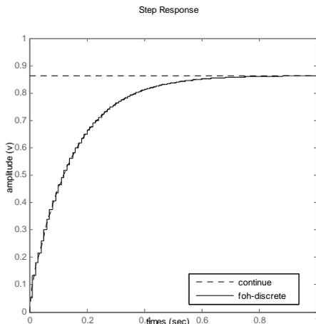
Figure 6. Step response of discrete system with FOH method
