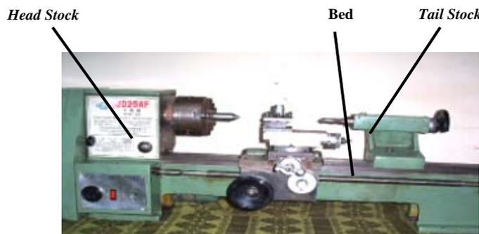
Figure 3. The Experimental Setup of a Spindle
