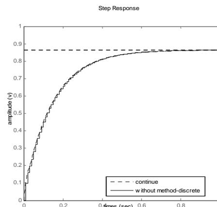
Figure 5. Step response of discrete system without method
