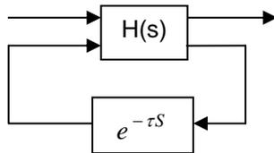
Figure 1. An internal delay
