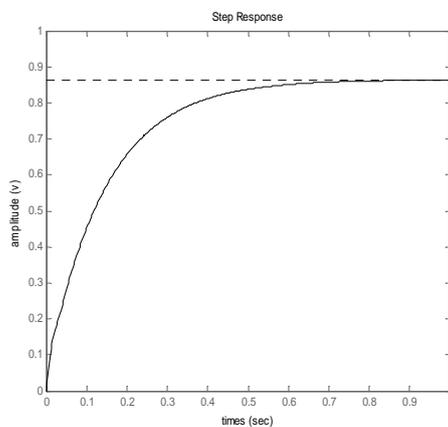
Figure 4. Step response of continuous spindle system
