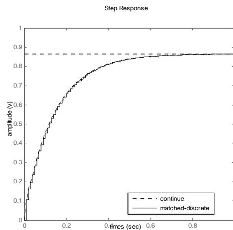
Figure 9. Step response of discrete system with matched method
