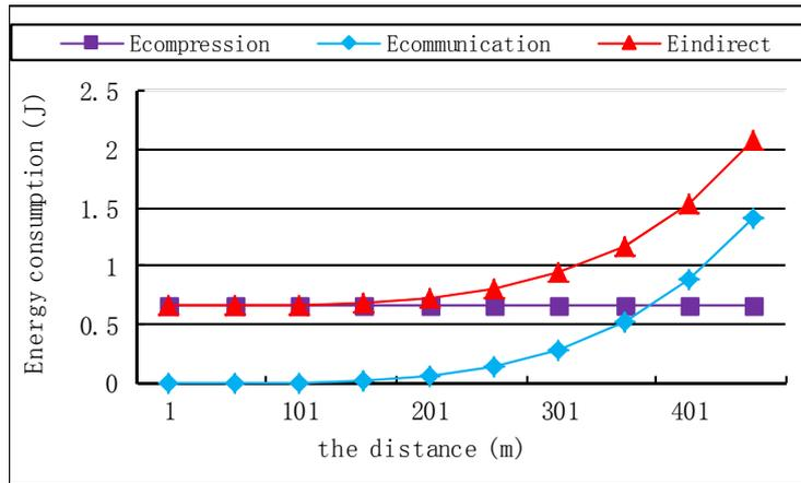
Figure 2. Energy consumption distribution of image compression and transmission
