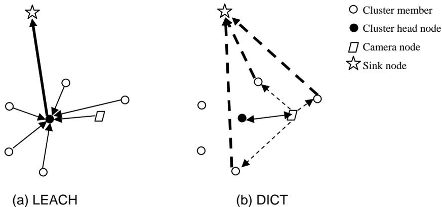
Figure 3. The data transmission path
