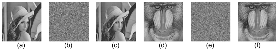
Figure 2. The results of Lena and Baboon. (a) Plain image; (b) Cipher image of (a); (c) Decrypted image; (d) Plain image; (e) Cipher image of (d); (f) Decrypted image.
