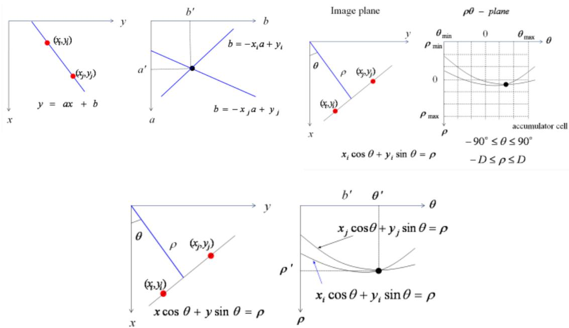
Figure 1. (a) slope-intercept equation; (b) normal representation; (c) Detecting lines via the HT
