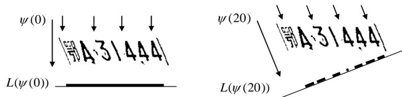
Figure 3. The different values of the projection function in different directions.
