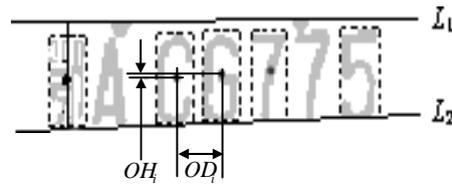
Figure 2. The geometrics configuration between neighboring characters.
