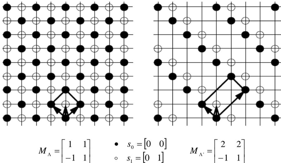
Figure 2: The lattice  $\Lambda$  is determined by the generator matrix  $M_\Lambda$ , 1-D filtering is applied along  $45^\circ$ . The generator matrix is  $M_{\Lambda'}$  after the sub-sampling, and the shift vectors is  $s_0$  and  $s_1$
