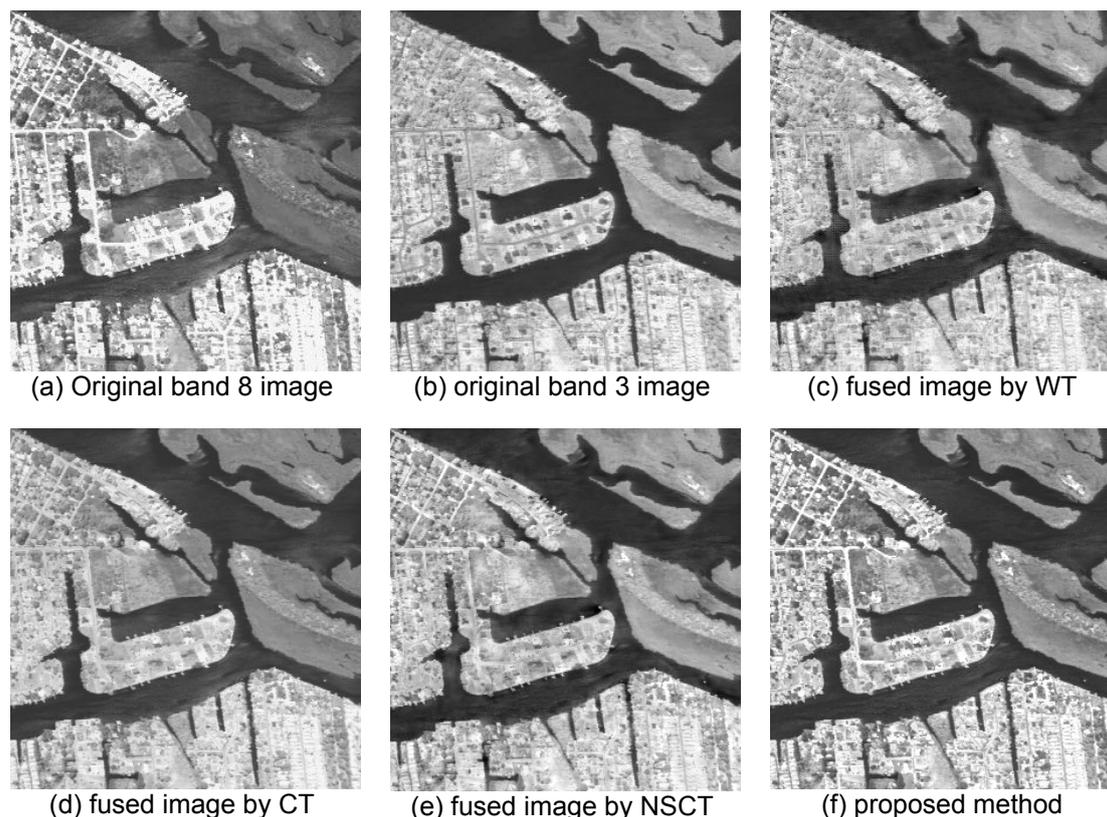
Figure 3. Fused image with the different methods. (a) Original band 8 image, (b) Original band 3 images, (c) fused image by WT, (d) fused image by CT, (e) fused image by NSCT, (f) Fused image with proposed method.
