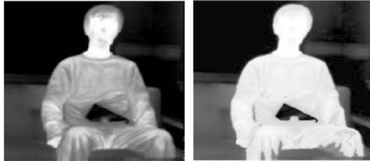
Figure 2. IR image before enhancement and after enhancement using MSR and Contrast Stretching
