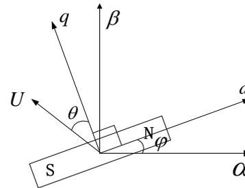
Figure 3. Vector control coordinate system
