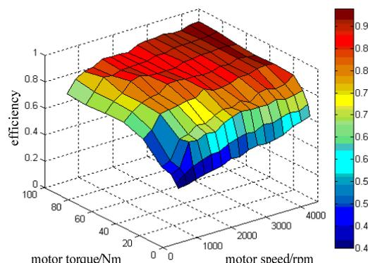
Figure 10. Motor efficiency graph
