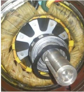
Figure 4. Prototype for the proposed FMDSPM
