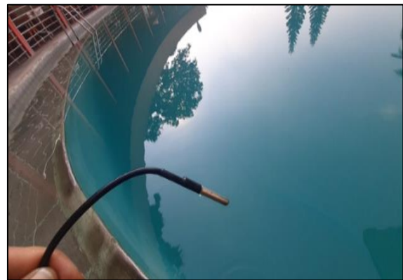
Figure 7. Temperature sensor to observe temperatures at different depths
