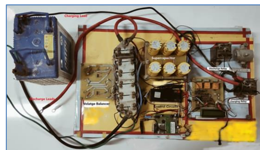
Figure 8. Hardware layout of developed HESS
