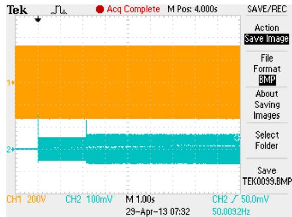
Figure 3. Experimental results after initial start of the on-grid inverter: Ch1 denotes the output voltage signal; Ch2 denotes the output current signal. The time span is (-5s,5s).
