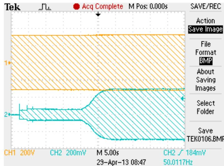
Figure 2. Experimental results after initial start of the on-grid inverter: Ch1 denotes the grid voltage; Ch2 denotes the output current signal. The time span is (-25s,25s).
