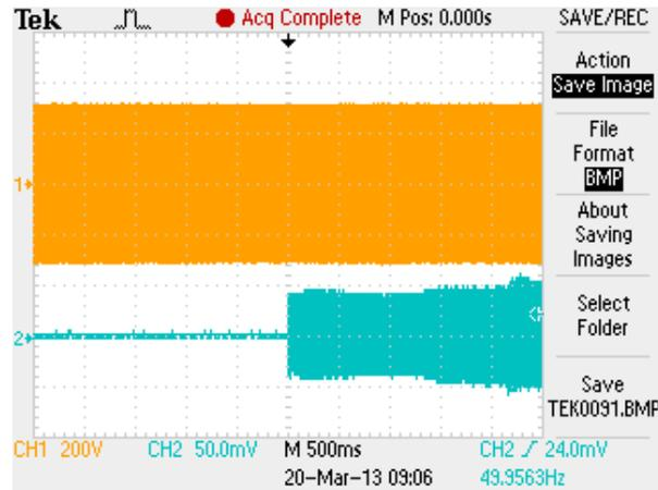
Figure 6. Experimental results after initial start of the on-grid inverter: Ch1 denotes the grid voltage; Ch2 denotes the output current signal. The time span is (-5s,5s).
