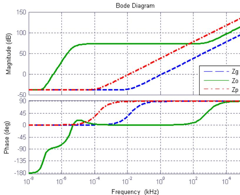
Figure 9. Frequency response of the inverter output impedance and the two different grid impedances
