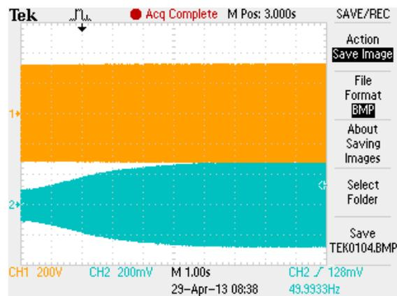
Figure 4. Experimental results after initial start of the on-grid inverter: Ch1 denotes the grid voltage; Ch2 denotes the output current signal. The time span is (-5s,5s).
