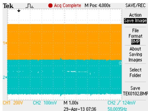
Figure 5. Experimental results after initial start of the on-grid inverter: Ch1 denotes the grid voltage; Ch2 denotes the output current signal. The time span is (-5s,5s).
