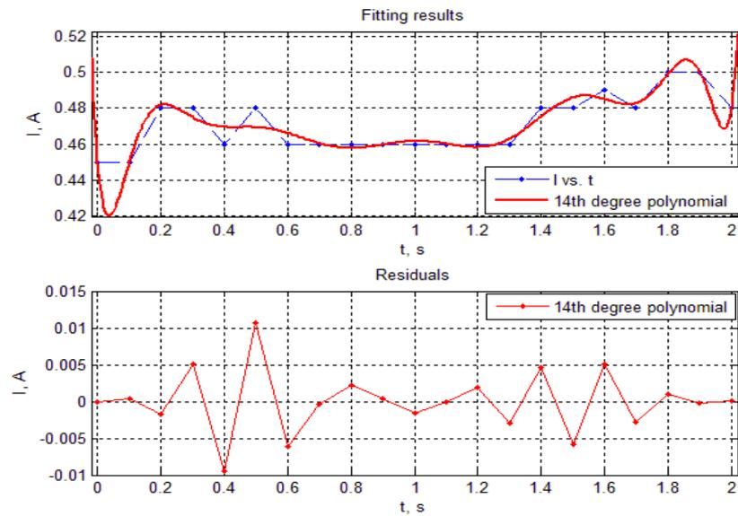
Figure 7. Simulation results of the fitting of the curve of the inverter output current I
