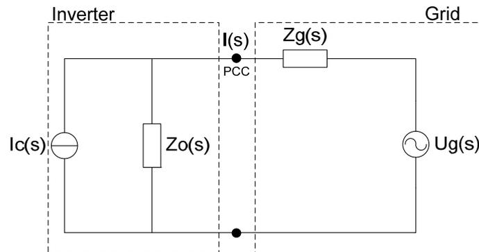
Figure 1. Norton equivalent circuit of on-grid inverter
