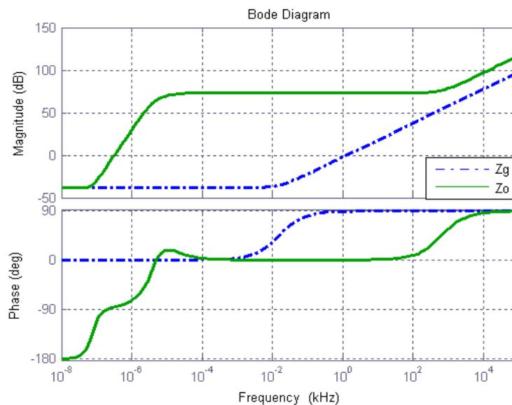
Figure 8. Frequency response of the inverter output impedance and the grid impedance
